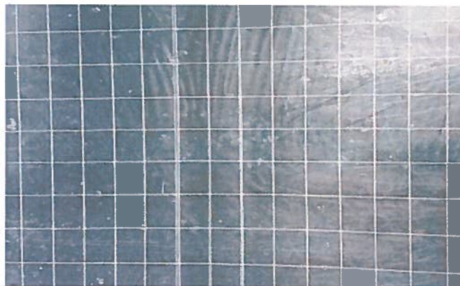
Product after 60 min of agitation in slosh box (on a 25 mm grid)
